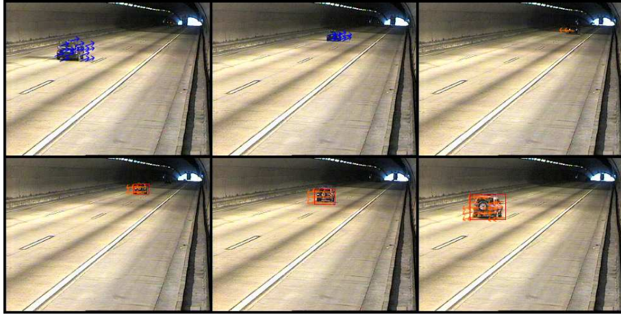
Fig. 9. Wrong way driver detection in a simulated event video sequence in a tunnel.
