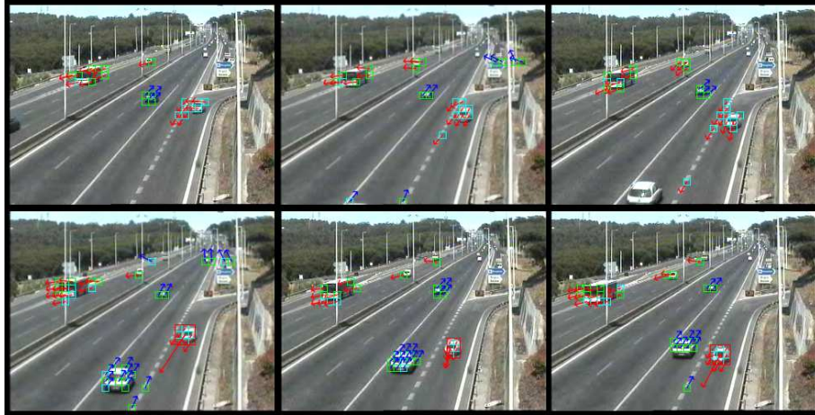
Fig. 8. Wrong way driver detection on simulated event video sequence. In the first three frames of the sequence, the vehicle entering the highway through the exit lane is being validated and then it is detected as a wrong way driver.
