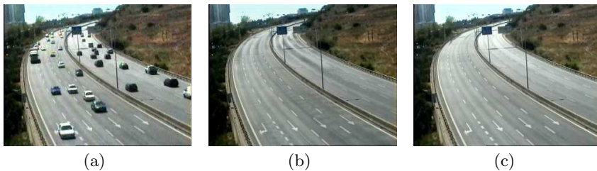
Fig. 1. Estimation of the initial background model. a) a frame of the scene where background model was computed. b) background model estimation with an weighted average of 500 frames; c) background model estimation with the median of 50 frames
