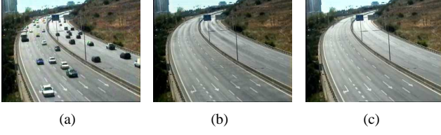
Fig. 1. Estimation of the initial background model. a) a frame of the scene where background model was computed. b) background model estimation with an weighted average of 500 frames; c) background model estimation with the median of 50 frames. As one can see, the weighted average estimation is darker in the regions where there is a higher number of vehicles passing (top of the road).
