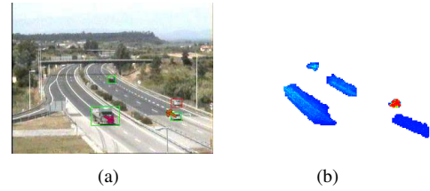
Figure 2. Stopped vehicles detection system experiments. a) stopped vehicle detection (red box); b) chromatic representation of the number of occurrences of the most frequent Codeword.
