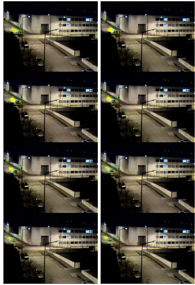
Fig. 5. Vehicle detection and tracking on a real night urban scenario.
