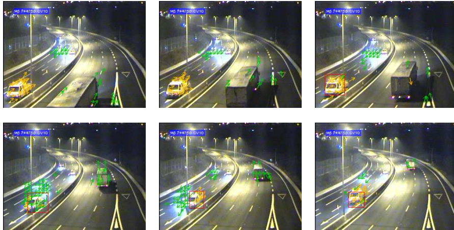
Figure 3.11: Wrong way vehicle detection at night. The vehicle is reversing in a lane disabled for maintenance.
