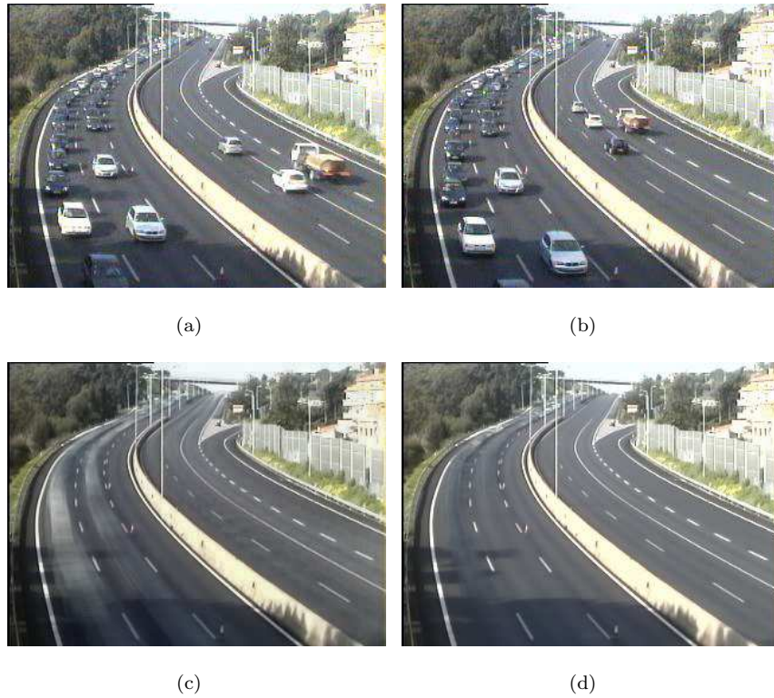
Figure 2.5: Initial background model estimation with traffic jam situation. a) and b) two frames of the scene where background model was computed. c) background model estimation with a weighted average of 500 frames; d) background model estimation with the median of 200 frames
