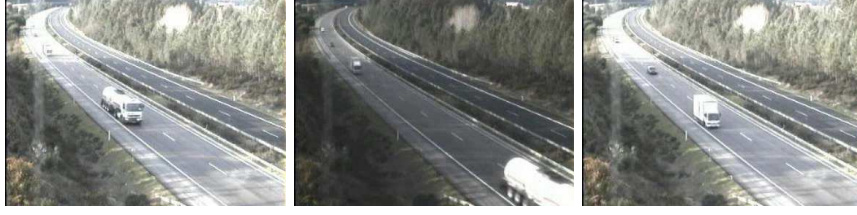
Figure 2.9: The camera's AGC changes the image brightness because of the truck that is coming towards the camera.
