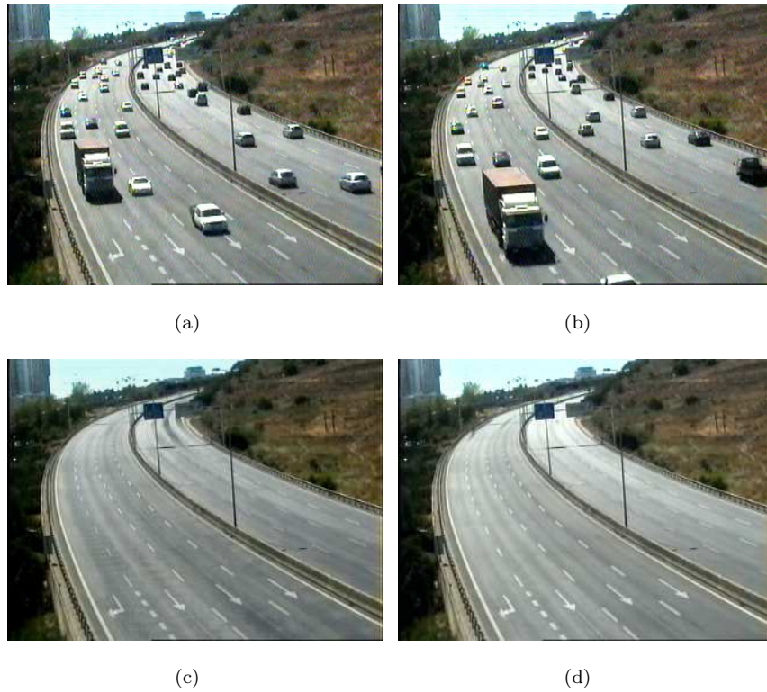
Figure 2.4: Initial background model estimation. a) and b) two frames of the scene where background model was computed. c) background model estimation with a weighted average of 500 frames; d) background model estimation with the median of 50 frames
