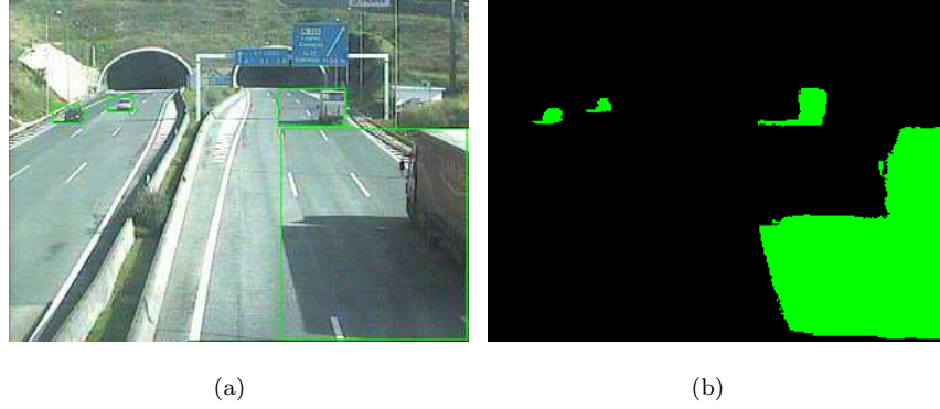
Figure 2.11: Example of a shadow problem in an outdoor scenario, the vehicle's shape and area change significantly. a) Bounding box of the vehicles detected with the proposed segmentation system. b) Foreground pixels detected with the proposed segmentation system (green pixels).
