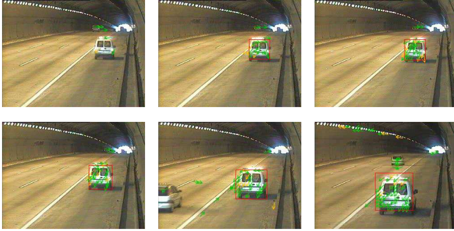
Figure 3.10: Wrong way vehicle detection in a tunnel scenario. The vehicle is reversing in the hard shoulder.
