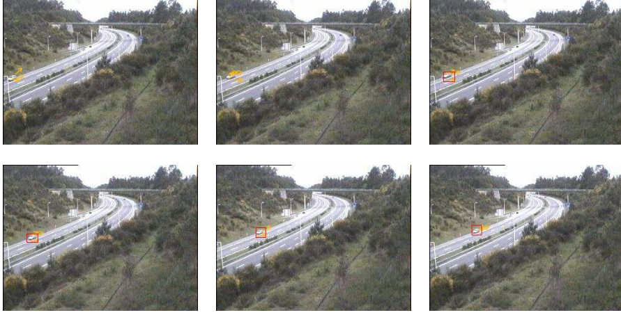
Figure 3.9: Wrong way vehicle detection in a typical outdoor scenario. The vehicle is reversing in the hard shoulder.
